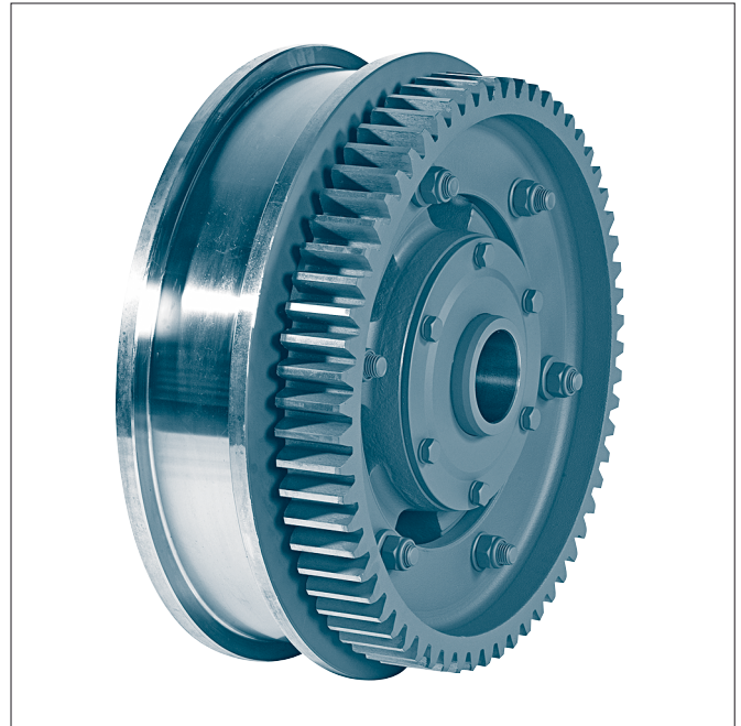
Form BG broad crane wheel with large gear ring (running surface- \varnothing d1 \geq 630 mm) gear ring screwed on
