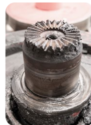
Example of gear profile reconditioning
