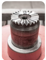
Example of gear profile reconditioning
