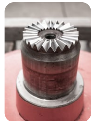
Example of gear profile reconditioning
