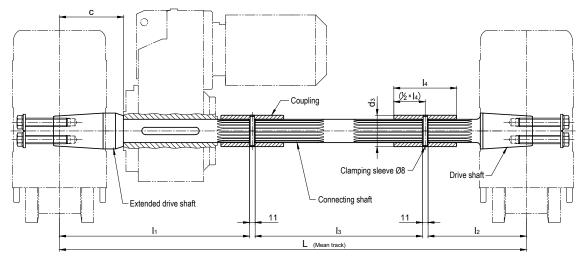
For gearboxes with hollow shaft and feather key connection in acc. with DIN 6885
