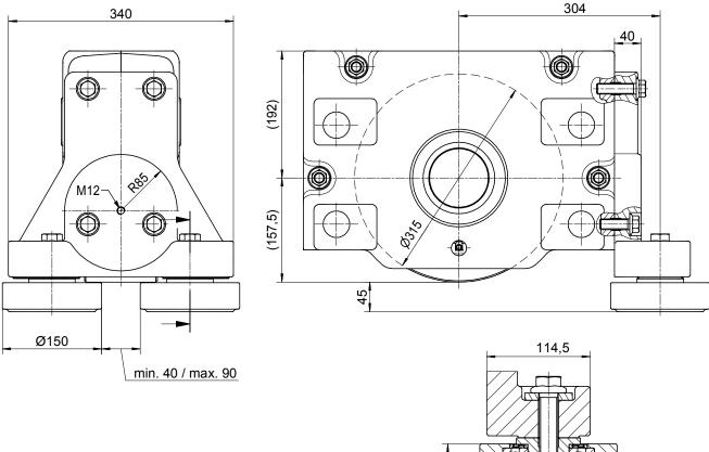
Acceptable horizontal load: Max. 3300 kg (As single part max. 4400 kg) ¢130
