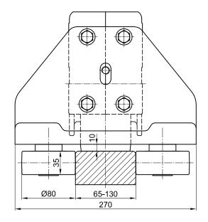
Magnified detail drawing of the guide roller
