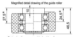
By turning the unsymmetrical guide roller, two clearances\* can be adjusted.
